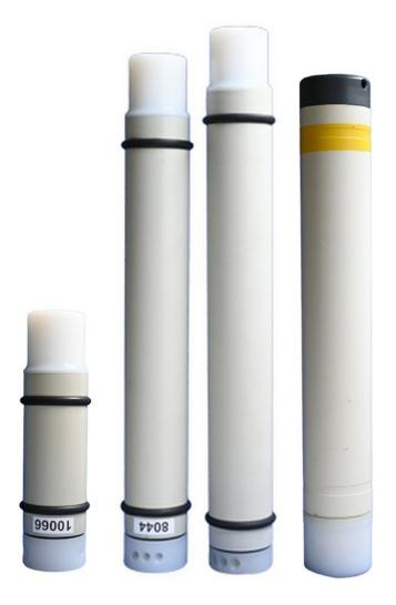
'Little' = LF-POD, Standard F-POD, Lithium Rechargeable F-POD, Deep F-POD The LF-POD will be replaced by a slightly longer lithium rechargeable version with a longer running time. The F-POD and C-POD can be immersed to 100m, Deep PODs can be immersed to 2000m. The Deep F-POD has a 3mm thick silicone rubber sheath, not shown.
