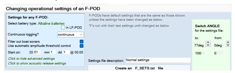
Select battery type: click the label to go through the options. This sets a minimum voltage for a stack of batteries, at which the POD will shift to the next stack on its list. The list starts with the weakest usable stack, so weak batteries are exhausted first in order to minimise discarding of part-used batteries.
