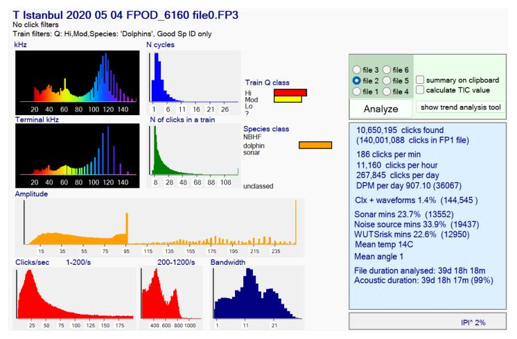
If an FP1 file is analysed the last entry in the results list is how long it would take to fill a 32GB SD card at the rate found.
