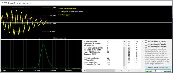
The data stored was the amplitude and timing (to 250ns resolution) of the peak of each wave shown. The waveform, in yellow, has been constructed by fitting sine waves to the 10 points stored. This synthetic waveform has been sampled at 1m samples per second to provide the input data for the Fast Fourier Transform (FFT) that gives us the frequency spectrum, shown in green. The data has been expanded to 512 samples by zero-padding at each end.
